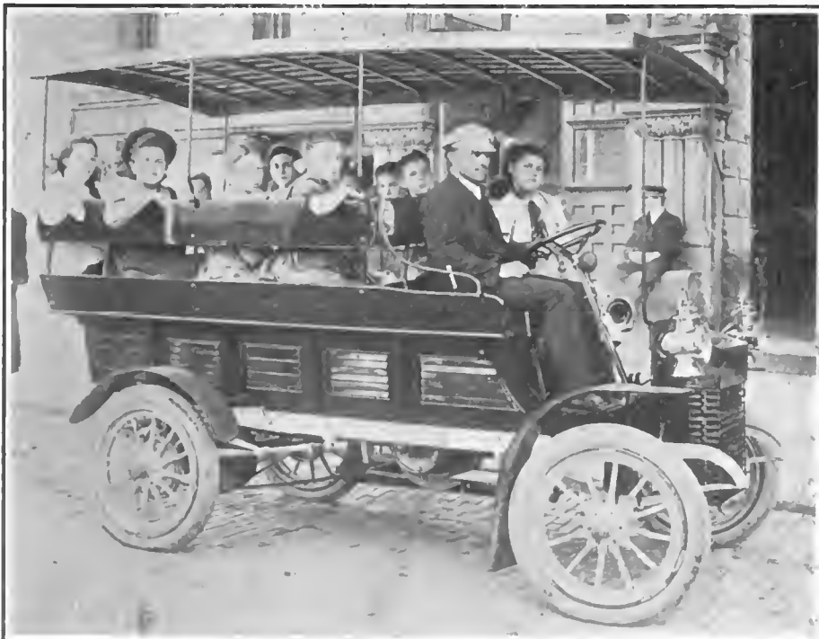
REO TEN-PASSENGER 16-H.P. OMNIBUS DRIVEN BY DOUBLE-OPPOSED ENGINE.
